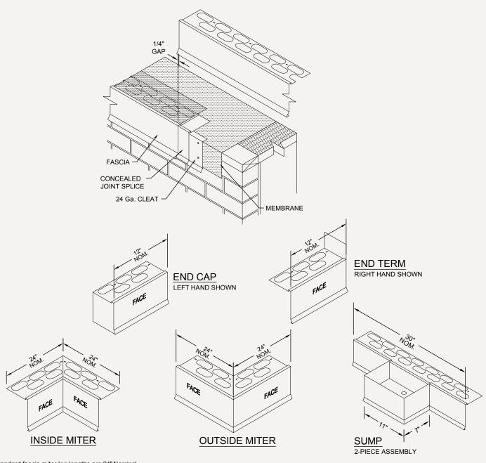
Standard fascia miter leg lengths are 24" Nominal Standard fascia miter angle is 90° For special miter requirements, attach sketches or consult manufacturer for assistance.
